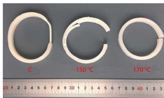
Fig. 5 Fracture specimens of the rotational PE pipes after tension. From left to right are the conventional pipe, the rotational PE pipe at 150 °C, and the rotational PE pipe at 170 °C.
